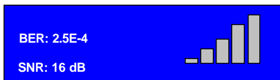
Figure 3 Off-Air Signal Diagnostics
